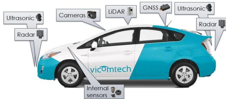
**Fig. 1.** Frequent sensors self-driving research vehicles are equipped with.
